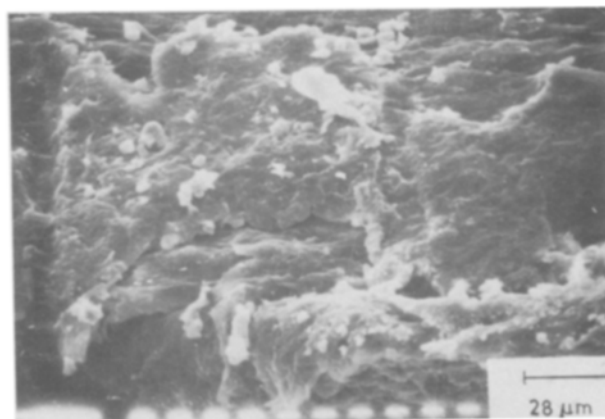
Figure 17 Abraded surface of E 50 d showing cracks and deformed matrix.
